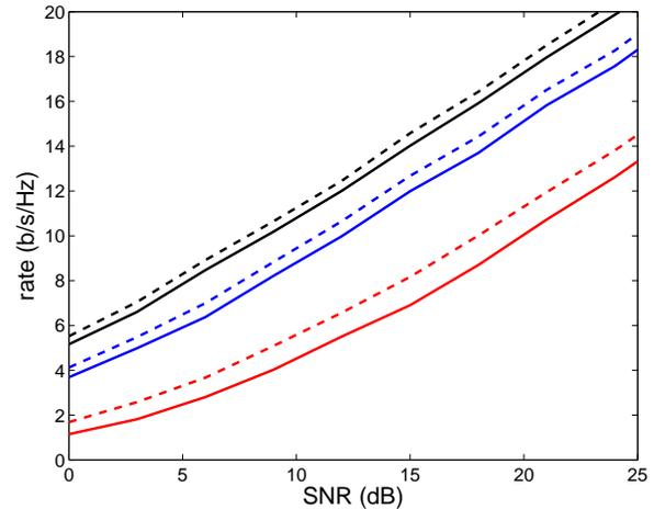
Fig. 2. Average MIMO-SNQ performance over random  $2 \times 2$  MIMO channel with spatio-temporal uncorrelated Gaussian scattering. The successively higher solid curves correspond to 1, 5, and 10 taps of ISI, respectively, and the associated dashed curves indicate the corresponding capacities.
