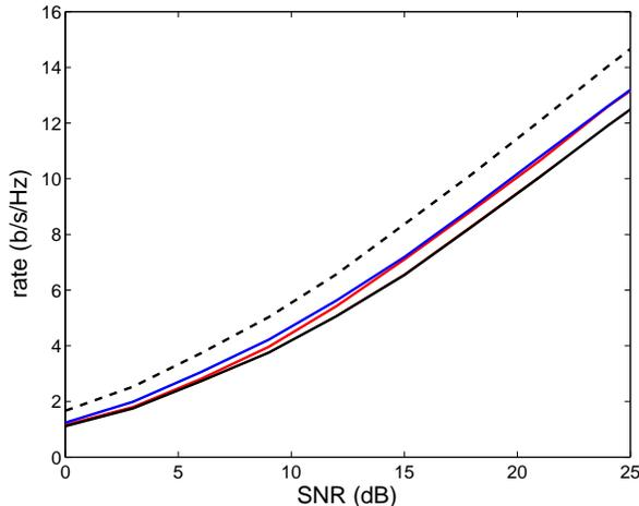
Fig. 1. Average MIMO-SNQ performance over random  $2 \times 2$  MIMO channels without temporal ISI. The successively higher solid curves correspond to V-BLAST with fixed-order decoding, MIMO-SNQ, and V-BLAST with optimum-order decoding, and the dashed curve indicates capacity.
