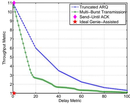
Fig. 3. The delay-throughput tradeoff for optimized MBT and truncated ARQ, compared to the genie-assisted bound and to the SUA scheme. ARQ performance is not shown, since it yields  $DM = \infty$ . Channel is i.i.d. with  $\rho = 0.5$  and  $d_c = 10$ .
