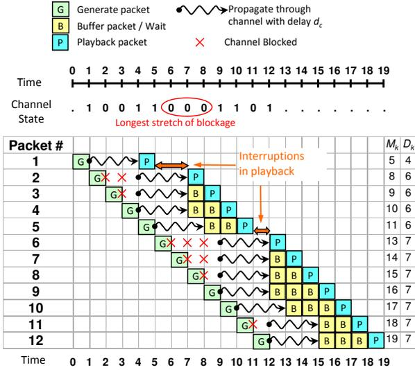
Fig. 2. Example of genie-assisted system operation with  $d_c = 3$ .
