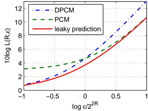
Figure 3: DPCM, PCM, and one-tap leaky prediction performance compared for an AR(1) source with  $\alpha_1 = 0.7$ ,  $R = 3$ . The critical error threshold is nearly  $\epsilon_0(R) = 2^{-2R}$ .
