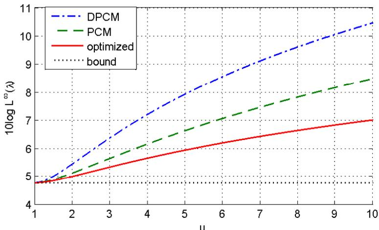
Figure 4: Performance comparison ( $\lambda = 2$ ) between three systems and the bound of (8), for sources in Example 3. The performance gaps from both DPCM or PCM to the system with optimized parameters is unbounded when  $u$  is taken arbitrarily large.
