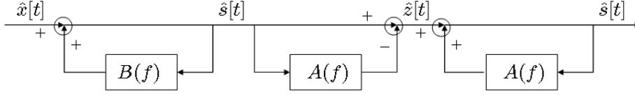
Figure 5: The equivalent system at the decoder. When a sample is not erased, the entire decoder implements  $1/(1-B(f))$ . When a sample is erased, the first two filters are effectively bypassed as the decoder sets  $\hat{z}[t]$  to 0.
