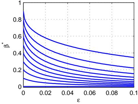
Figure 2: Encoder predictor  $\beta_1 = \beta^*$  that minimizes  $D_{\text{leaky}}(R; \epsilon)$  for  $R = 3$  bits/sample and various values of  $\alpha_1 = \{0, 0.1, 0.2, \dots, 0.9\}$  (bottom to top).
